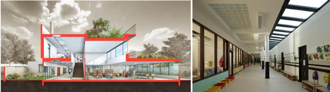
Figure 7. Left: cross section of the school in Limeil-Brevannes with the playground on the roof and the large bay windows to bring daylight in the classrooms and the library. Right: Picture of the glass cobblestones integrated in the circulation on the first floor. Source: http://www.ekopolis.fr
