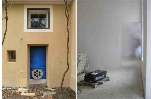
figure 16: Blower Door test with smoke test, done during construction phase (c) Manuel Benedikter
